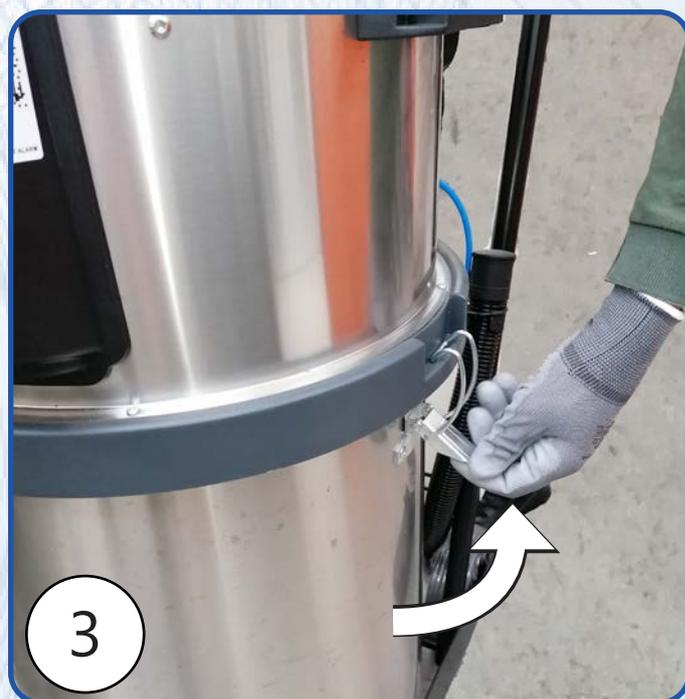
④ Lift the upper part of the steel drum and position it so that the drainball valve can be easily reached. Open with carefully the drainball valve in order to drain away any water inside it through the pipe which must be placed inside a container.
