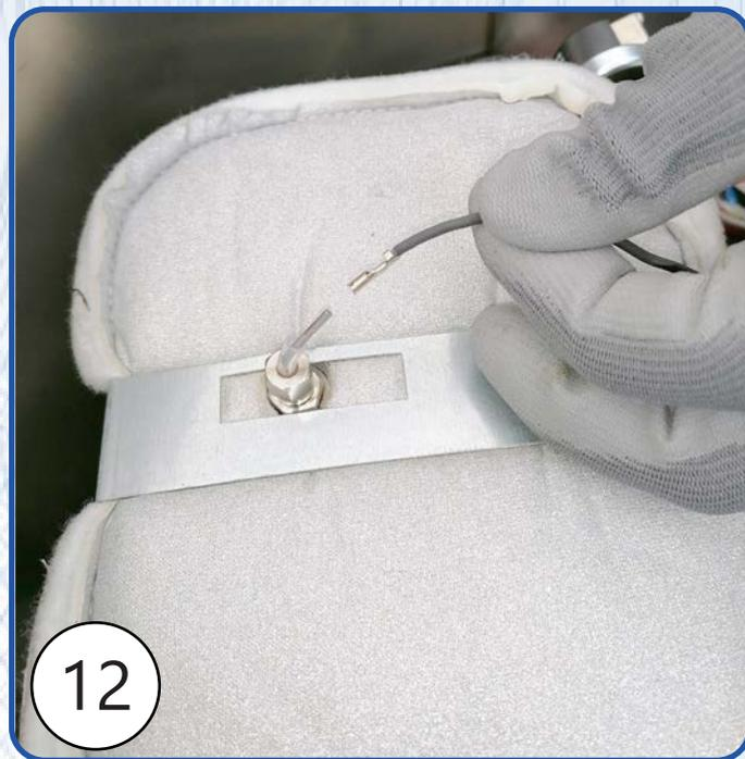
⑬ Disconnect the two cables connected to the pressure switch.
